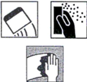
~~*New iron:* Make sure that the substrate is perfectly dry and free from traces of grease and oil. Otherwise, clean the surface with solvent or an appropriate degreaser. With the steel brush or the abrasive paper, remove the calamine and the rust where present; finally clean the surfaces to be painted. Then apply two coats of anti-rusting PROTEZIONE 3 and after 12-24 hours coat with two coats of FLAVIA BABY following the technical instructions below.~~
