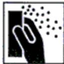
Prepare the surface with powder or pasty putty as (such as Flystuk). After about 12 hours from the end of the application treat with abrasive papers: It is recommended a grain type P120. Apply 1 coat of acrylic fixative FISSACRIL diluted with water 1:1/1:3. After 4-5 hours apply - by a roller - 2 coats of UNIVERSAL PRIMER at an interval of 5-6 hours from one another. The Primer has to be colored in the same shade of the decoration to realize: VELLUTO FIORENTINO
