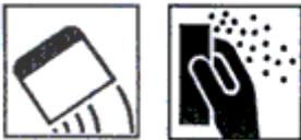
*New timber or trim:* All surfaces must be dry and seasoned. Rough surfaces can be filled with putty FLYSTUK to provide a smooth surface; Ensure the support to be coated is clean with dust and dirt removed. Then apply two or more coats of LEGNO NUOVO OPACO. For the application please refer to the technical methods given below.
